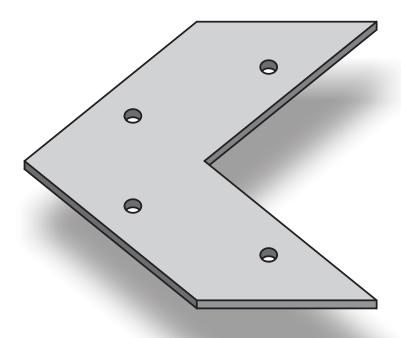
The Corner Key has pre-punched holes to allow for fast and easy assembly using our self-drilling screws, part #5217. The holes do not affect the functionality or structural integrity of the Corner Key. The Corner Keys are tumbled for easy insertion and accommodate mechanical fastening, welding, or bonding assembly.
